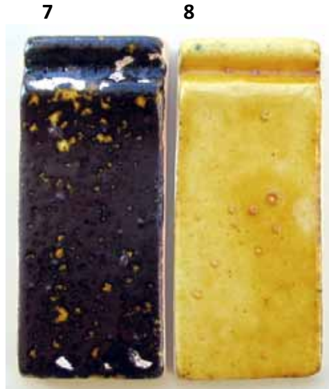
Şekil 27. Kil-sülyen-kalsine boraks 1040°C Figure 27. Clay-Red Lead-Calcined Borax 1040°C
