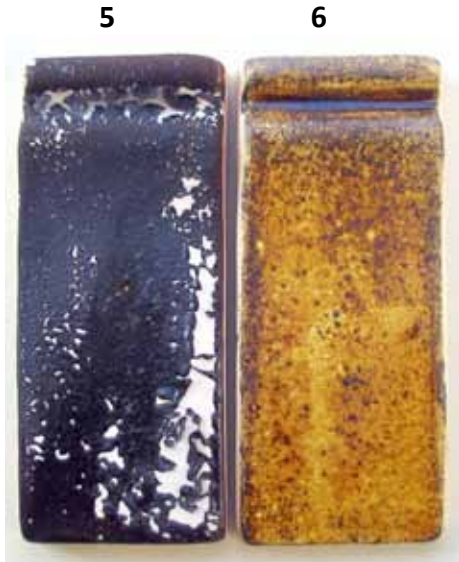
Şekil 26. Kil-sülyen-kalsine soda 1040°C Figure 26. Clay-Red lead-Calcined Soda 1040°C
