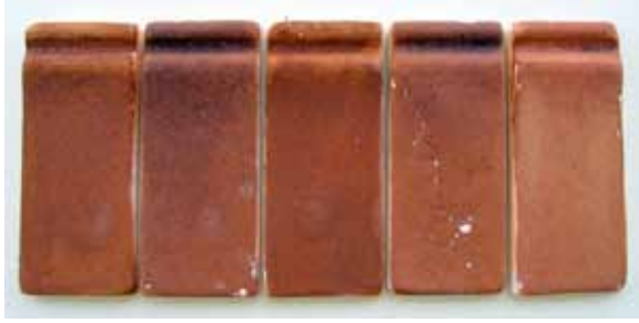
Şekil 6. Kil - Potas denemeleri 1040°C Figure 6. the test of Clay – Potash 1040 °C
