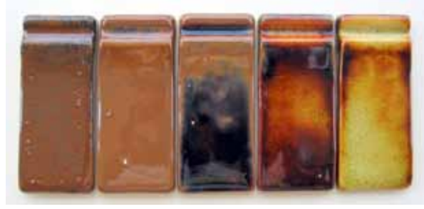
Şekil 19. Kil – kalsine Boraks denemeleri 1250°C Figure 13. The test of Clay – Calcined Borax 1250 °C
