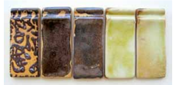
Şekil 17. Kil – kalsine Soda denemeleri 1250°C Figure 17. The test of Clay – Calcined Soda 1250 °C
