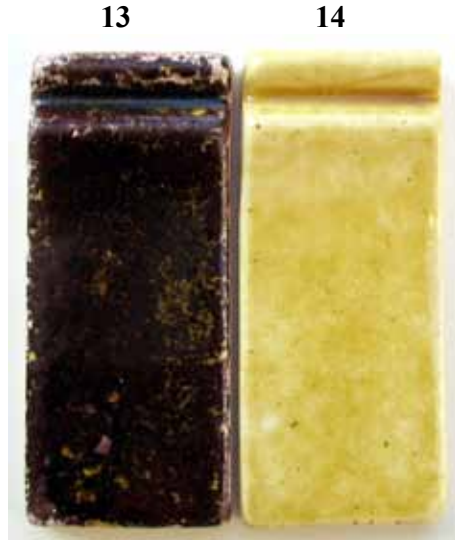
Şekil 30. Kil-kolemanit-kalsine boraks 1040°C Figure 30. Clay-Colemanite- C. Borax 1040°C
