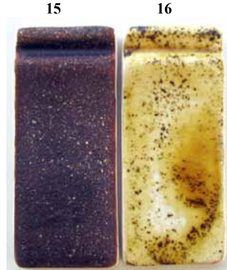
Şekil 31. Kil-üleksit-kalsine soda 1040°C Figure 31. Clay-Ulexide-Calcined Soda 1040° C
