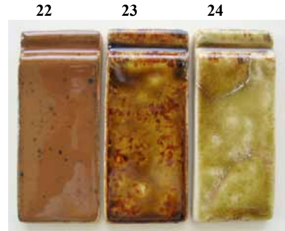
Şekil 41. Kil-üleksit-kalsine soda 1250°C Figure 41. Clay-Ulexide-Calcined Soda 1250°
