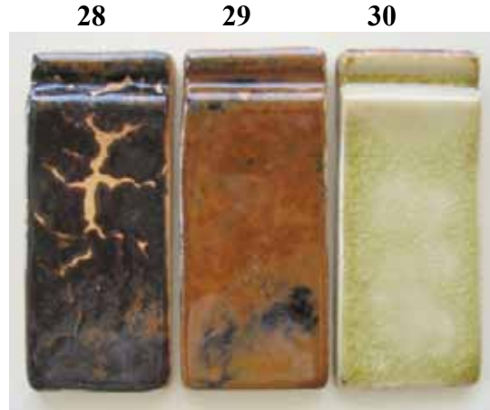
Şekil 43. Kil-kalsine soda-kalsine boraks 1250°C Figure 35. Clay-Calcined Soda-Calcined Borax 1250°
