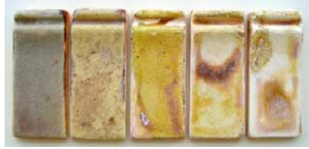
Şekil 7. Kil – Kalsine Soda denemeleri 1040°C Figure 7. The test of Clay – Calcined Soda 1040 °C
