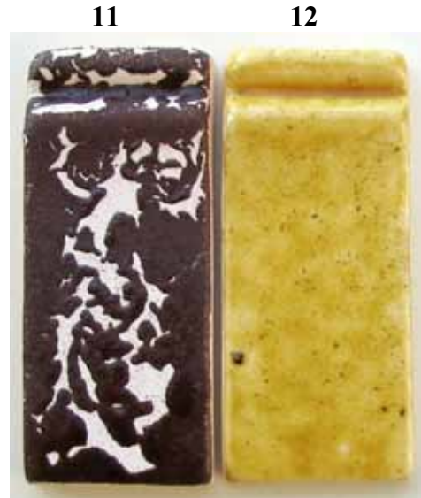
Şekil 29. Kil-kolemanit-kalsine soda 1040°C Figure 29. Clay-Colemanite-Calcined Soda 1040°C
