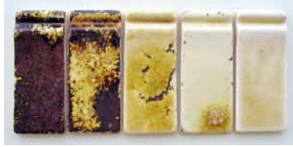
Şekil 9. Kil – Kalsine boraks denemeleri 1040°C Figure 9. The test of Clay – Calcined Borax 1040 °C
