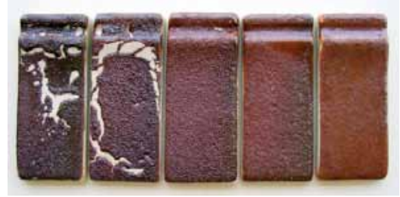
Şekil 13. Kil – Albit denemeleri 1250°C Figure 13. The test of Clay – Albite 1250 °C
