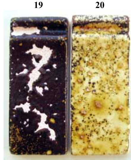
Şekil 33. Kil-kalsine soda-kalsine boraks 1040°C Figure 31. Clay-Calcined Soda- C. Borax 1040° C
