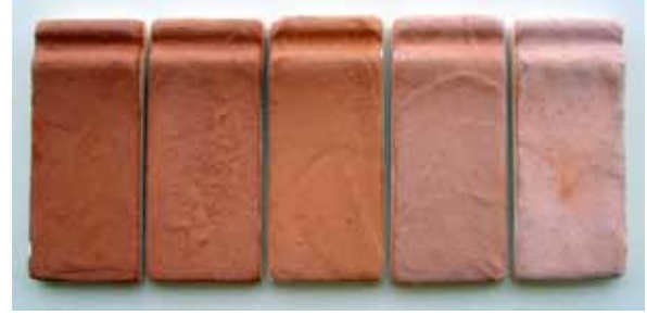
Şekil 3. Kil - Albit denemeleri 1040 °C Figure 3.the test of Clay – Albite 1040 °C
